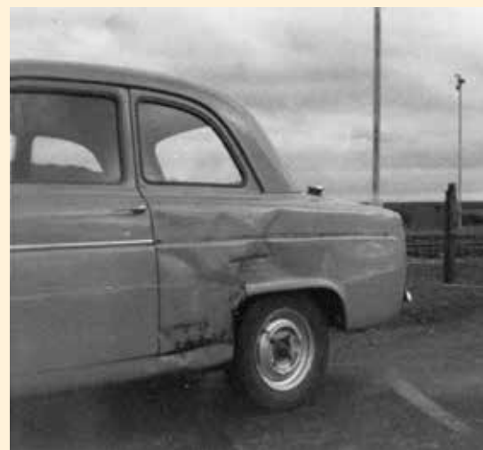
Yet further but more serious accident damage, this time requiring a new sill and quarter panel. The hazards of everyday use, I suppose.
