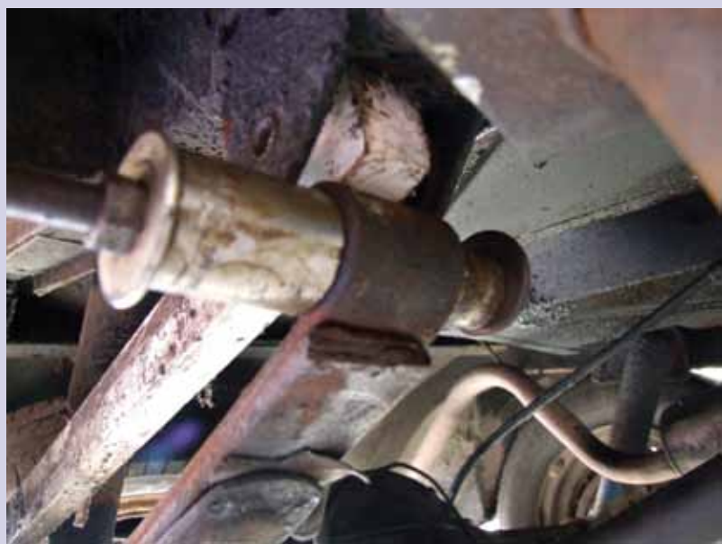
Photo 2. The front spring eye lowered and held down by a block of wood. The press tool consists of two sockets, two washers, one suitable stud and two nuts. Simple but effective!
