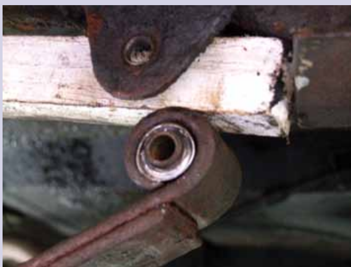
Photo 5. The new bush fully home. The inside tube is longer than the outer so the two-socket method must be used for installation as well as removal.
