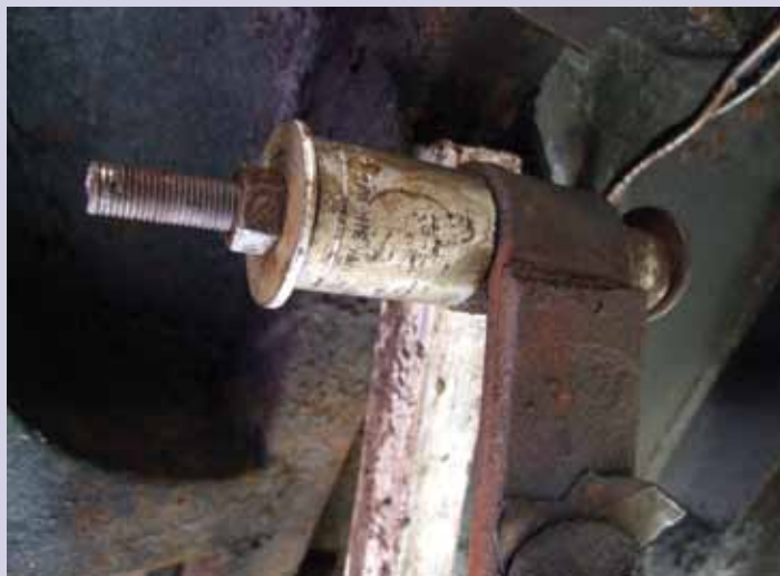
Photo 3. The bush about half way out, at which point it reached the end of the large socket, which was replaced by a deeper one.
