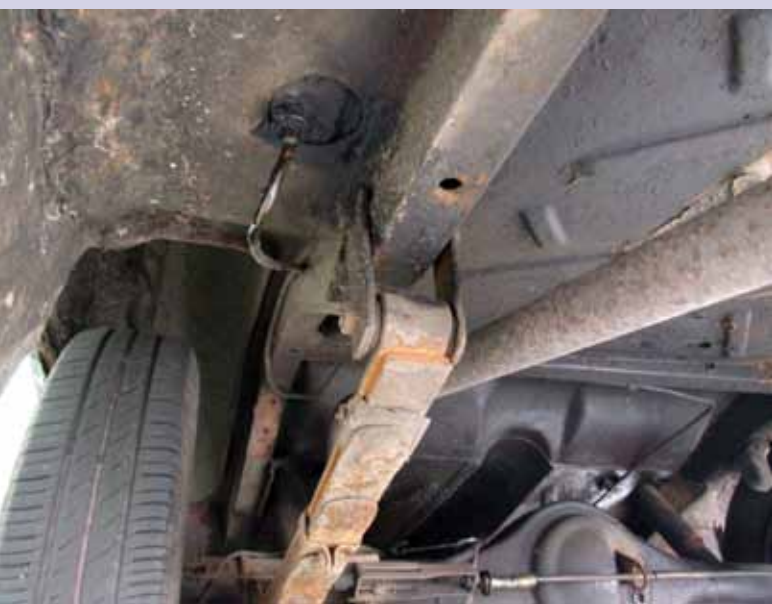
Photo 1. Under the rear of BLC, showing the spring shackle, wider at the top than the bottom. The dampness on the fuel pipe is releasing oil prior to a different job. The shackle has been fitted the opposite way around so that in future it can be removed inwards without fouling the fuel pipe.
