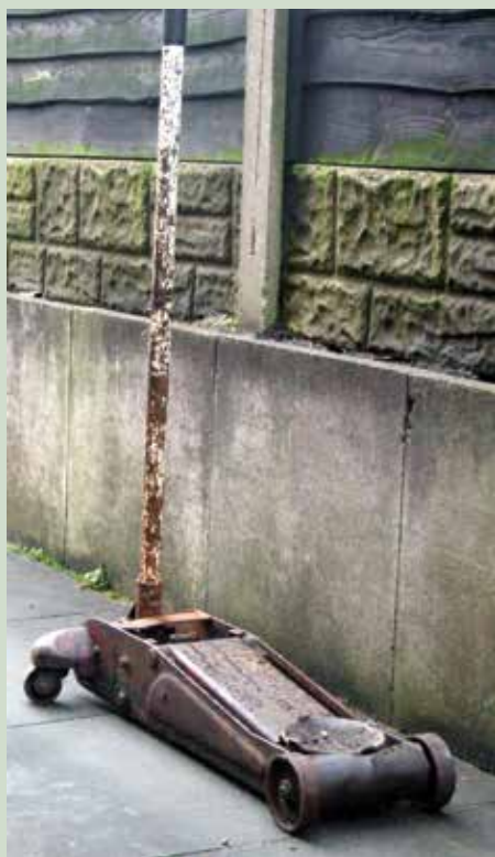
Photos 1 and 2: My own Bradbury 1½ Ton trolley jack, acquired secondhand many years ago and still giving good service. This is a professional standard jack, and its modern equivalent will be beyond the DIY mechanic. It has a lifting range of 4½" to 19".
