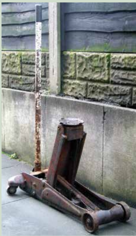
Photos 1 and 2: My own Bradbury 1½ Ton trolley jack, acquired secondhand many years ago and still giving good service. This is a professional standard jack, and its modern equivalent will be beyond the DIY mechanic. It has a lifting range of 4½" to 19".
