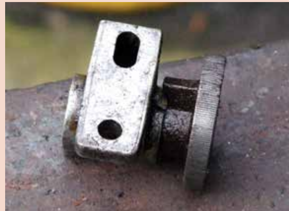
Photo 5. The original adjuster with the elongated hole. The serrations were intact on this part of the snail cam.
