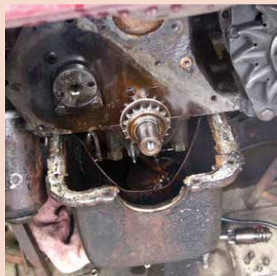
Photo 6. The adjuster removed. The cranked stud is to the left of the main bearing cap.
