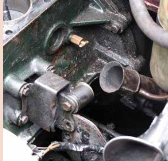
Photo 4. The socket doing a job for which it was never intended: maintaining the engine at a height above the crossmember.
