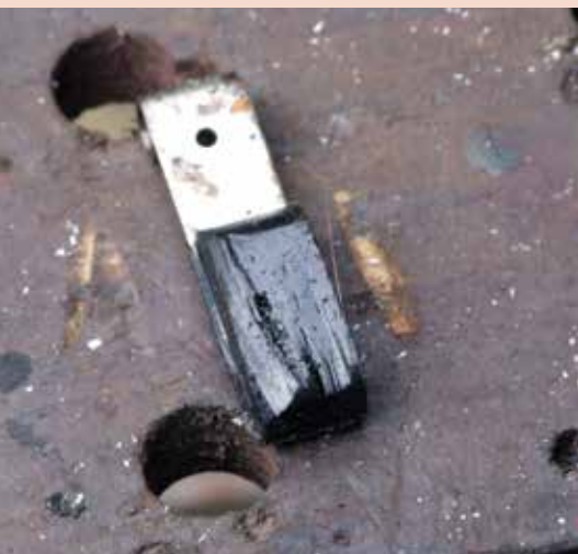
Photo 3. The badly worn adjuster pad.
