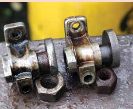
Photo 2. The original and replacement snail cams and the lack of serrations.
