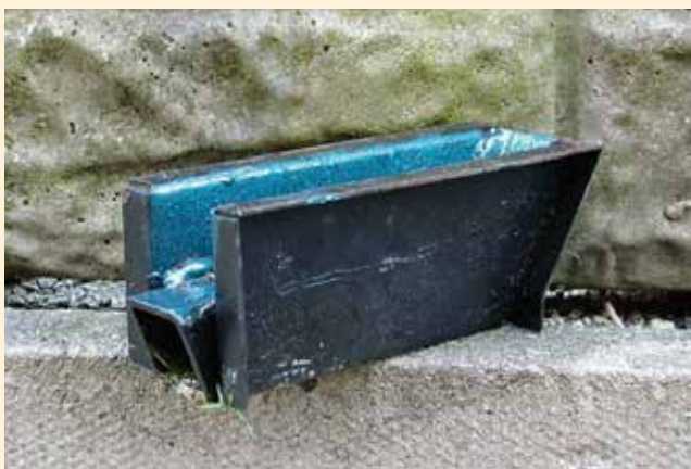
Photo 38. The new jacking point in its raw state. I could easily have made one, but not knowing how much time I had spare made it simpler to buy it off the shelf. The blue paint is Hammerite.
