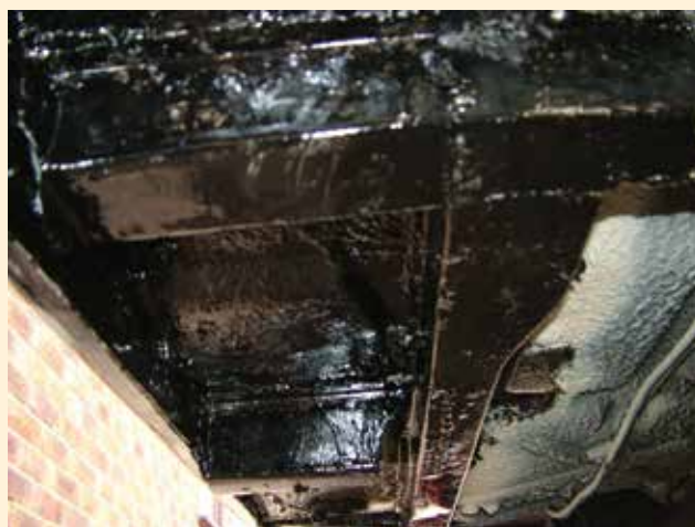
Photos 36 and 37. Underside view after painting, showing the jacking point part way along, while at the top is the front outrigger. This is fabricated from flat steel cut to size, with four parallel right angle bends put in as already described to form a top hat section.
