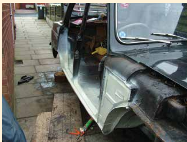
Photo 40. A look down the side of the car; the drive is narrow and this is the nearest to a side view available. The welding is complete and all new and repaired metal in primer paint, followed by top coat or black Hammerite as appropriate.
