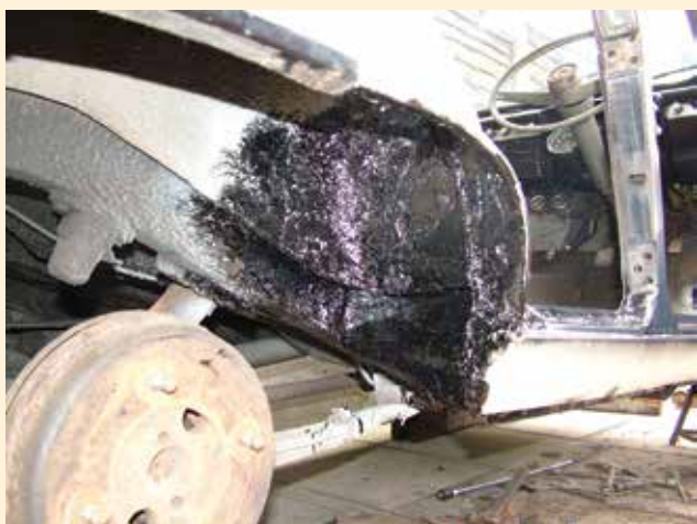
Photo 39. The triangular outrigger fitted very well. Although it could have been fabricated, it is a tricky piece to do and even Ex-pressed make it in two parts, then weld them together. Following the problem with the sill, I was very relieved at the good fit.
