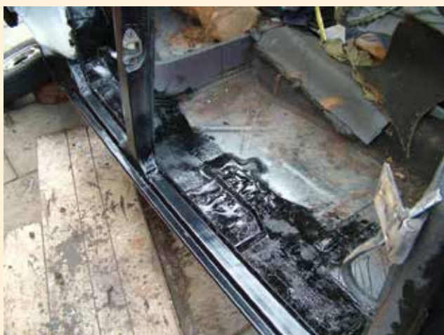
Photo 34 and 35. At the same time, the hole above the jacking point was repaired. This allowed the jacking point to be welded in, once suitable slots had been made in the sills' lower flanges to accommodate it.
