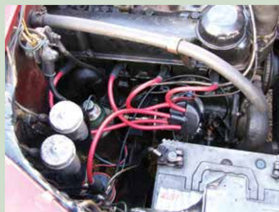
Photos 2 and 3. The system installed. Except that two L.T. leads leave the distributor, no-one would realise that this isn't the standard contact breaker system.
