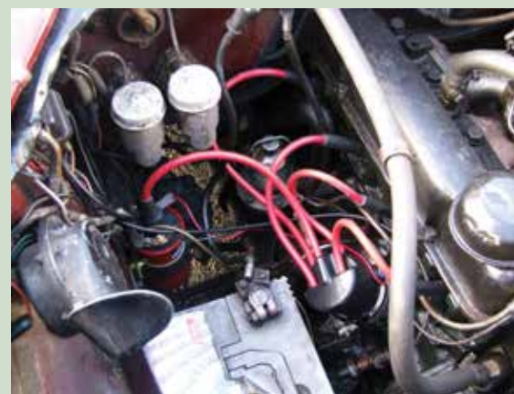
Photo 1. All the components as bought. The only modification needed was to trim the plug leads to length.
