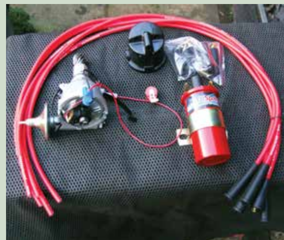
Photo 1. All the components as bought. The only modification needed was to trim the plug leads to length.
