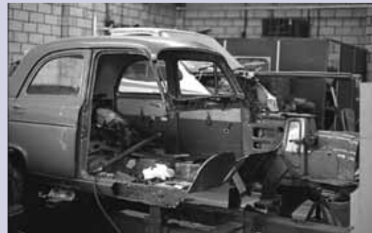
Photo 3. Despite massive damage, I decided to repair the car. It is here on the jig at work, and it will be realised just how much of the structure had to be replaced.
