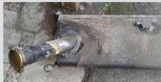
Leaking filler neck on upright fuel tank
