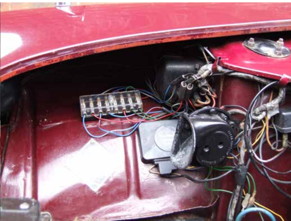
The fuse box and electronic ignition unit on the offside fitch panel. The wiring has been tidied up since the photo was taken.
