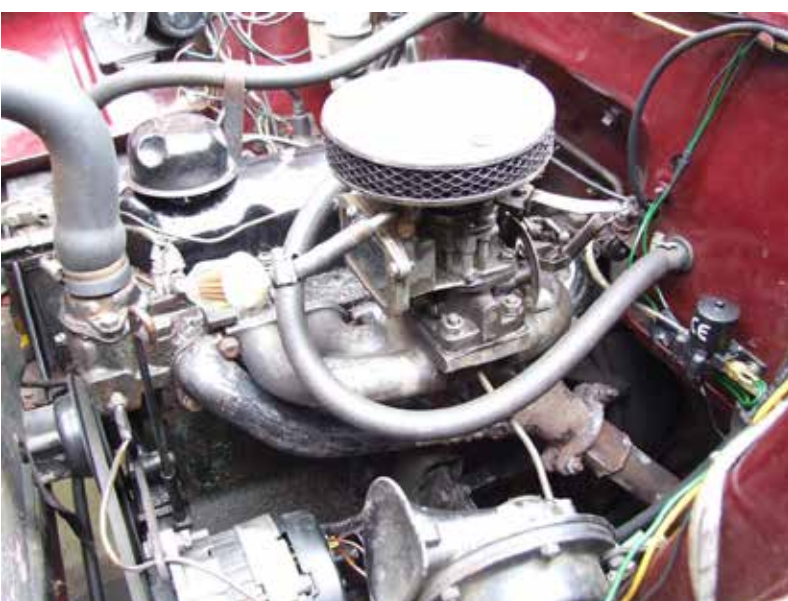
General view under the bonnet, showing manifold, alternator and screen wash pump.
