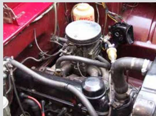
Nikki carburettor and manifold. The Lucas washer bottle is behind, positioned to receive heat in freezing weather. Just visible beyond are relays for the fog lamps and radiator fan.
