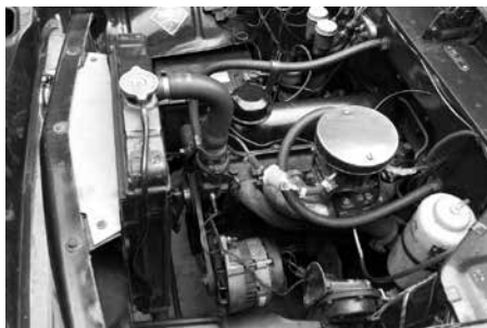
A view of the carburettor, manifold and washer bottle, as well as the alternator.
