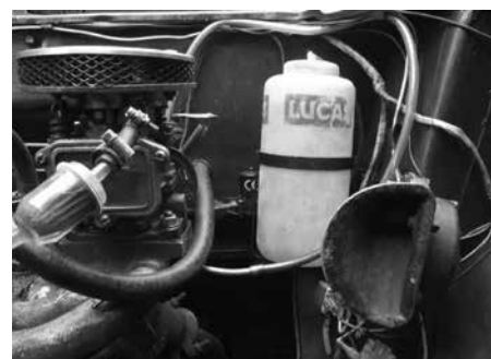
Another view of the carburettor, manifold and washer bottle, with the electric pump just visible.
