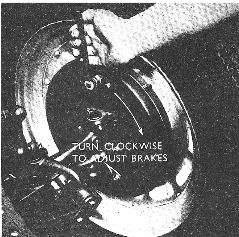
Adjusting brakes, upright.
