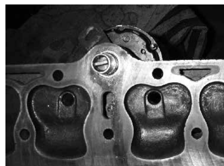
Bottom view: when you dare not hit the drive spindle there is not much area to work with.
