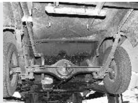
The original rear axle; there should be a bracket surrounding the handbrake rod, and the dampness of the banjo due to the leak is apparent. So too is the oil thrown around by the pinion flange.
