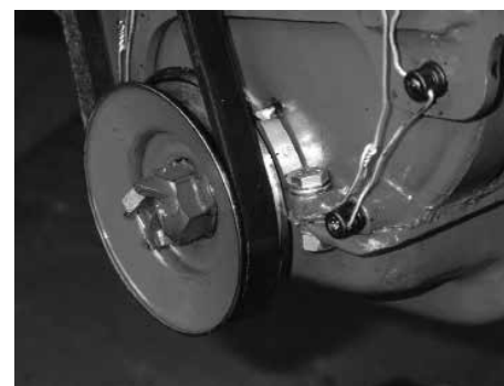
The brass timing scale used on my engine. The two notches are cut in its edge. The upper one adjacent to the white painted mark on the pulley is the ignition point and the lower one the top dead centre mark.
