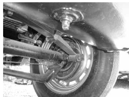
Driver's side, rear. Petrol tank and drain. Rear axle casing and wheel. Rear radius rod (hockey stick). Shock absorber arm and link. Brake cable and dust cover. Spring and shackle. Brake plate.
