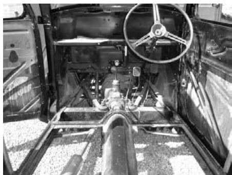
Front cross member. Gearbox casing and rear mountings onto cross member. Torque tube and universal joint casing. Handbrake and cable assembly. Rear of engine clutch housing. Brake and clutch pedals. Diagonal chassis support. Exhaust (just visible). N.B. wiring loom speedometer cable and gear not yet in place.
