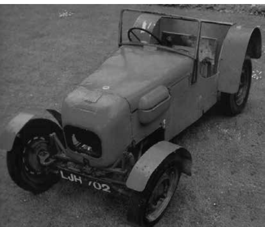
Lotus Mk II 3. SPORTS, with 1172cc Ford 100E tuned Sidevalve engine, drum brakes, live rear axle, framed windscreen and weather equipment for road use. Only seventeen Series 1 and ten Series 2 Lotus Elevens were fitted with Ford Sidevalve engines.
