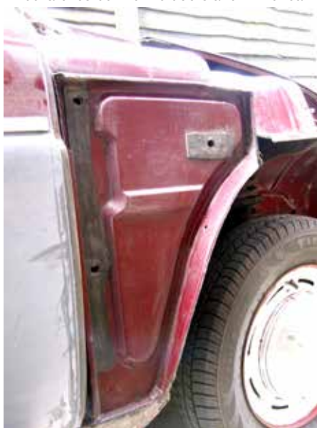
Left and right: O/S/F wing removed, again after a wipe with white spirit
