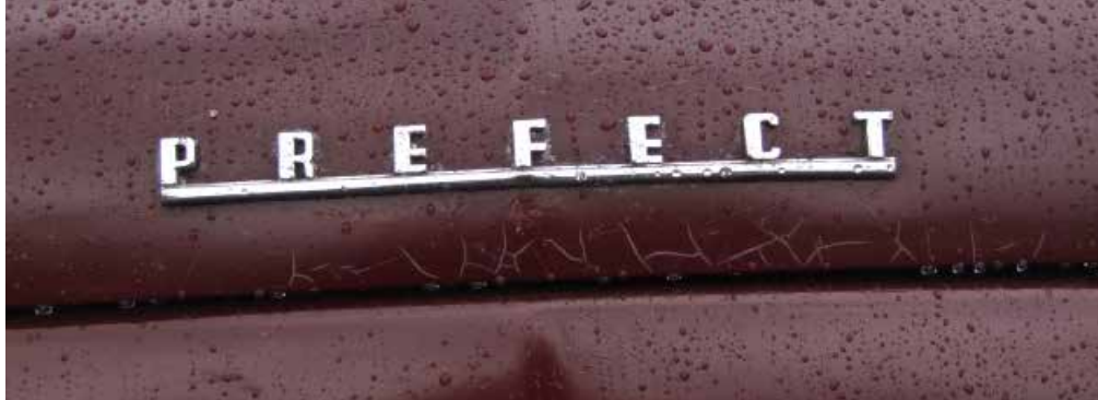
The cracking in the paint of the bonnet and front panel.
