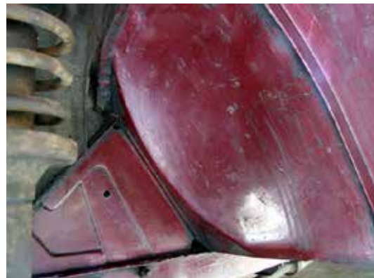
Inside the N/S/F wheel arch after no more than a wipe down with white spirit
