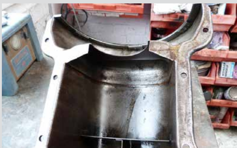
Right: thinners running through the brazed area.
