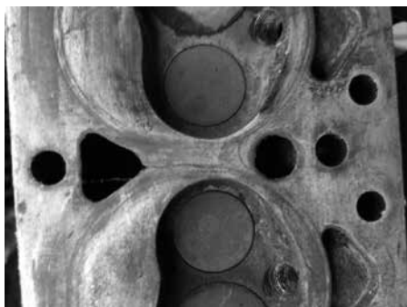
The crack across the head between Nos. 2 and 3 chambers. Unfortunately this is the Stage II head, so is now scrap.
