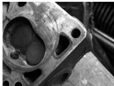
Wastage to the water passages at the rear of the head, allowing the cooling system to pressurise and expel the coolant past the filler cap.
