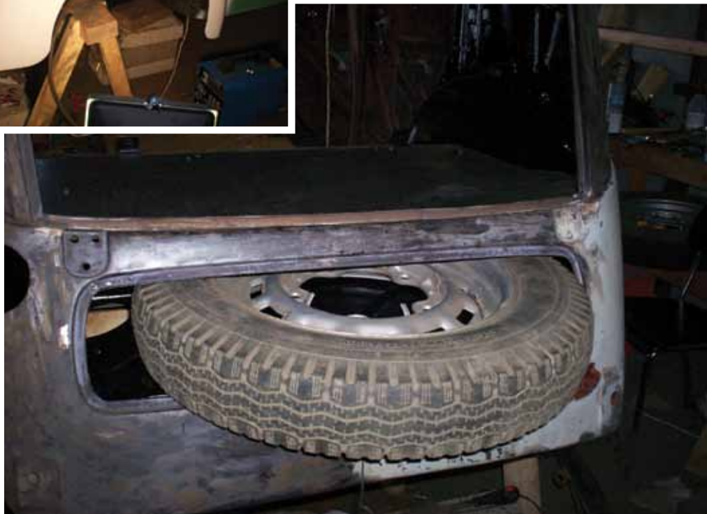
Winter grade tyres do not fit through the spare wheel opening in the Prefect. Photos by Håkon B. Øverland.
