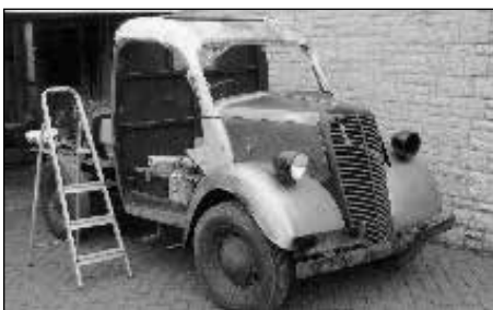
Picture 1: (above) MBW138 assembled to check panel fit before dismantling and painting.
